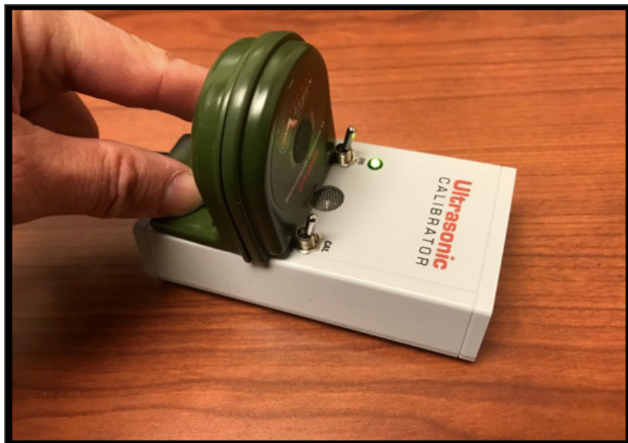
Figure 69. Hemidirectional microphone calibration. Image from Wildlife Acoustics
