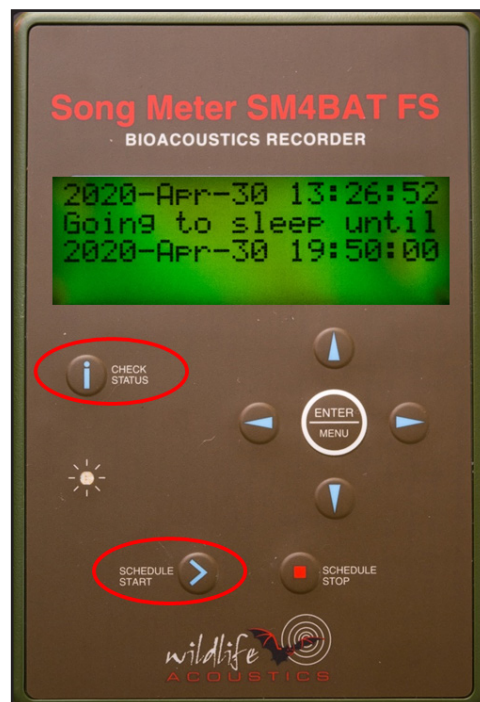
Figure 72. Select the “SCHEDULE START” button and the detector will go to sleep again (Step 4).
